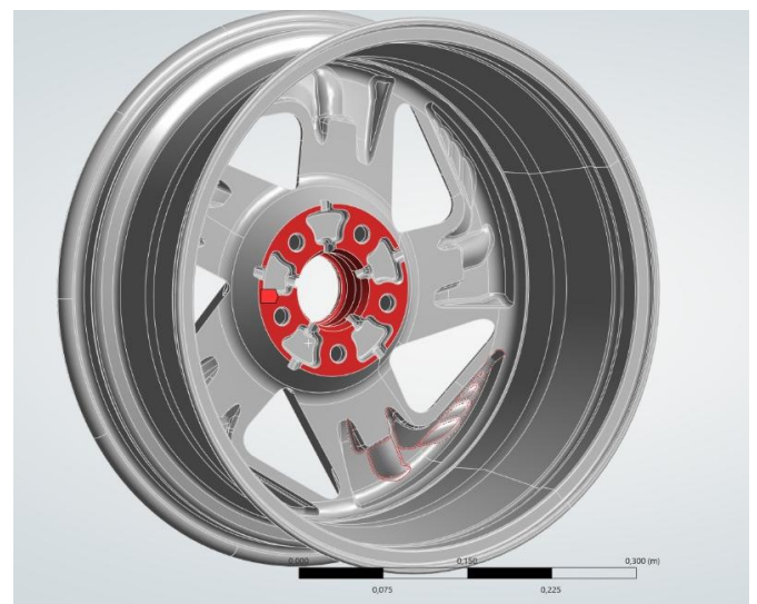
Figura 4.4: (a) Dettagli Fixed-Back; (b) zone modello appartenenti a Fixed-Back
