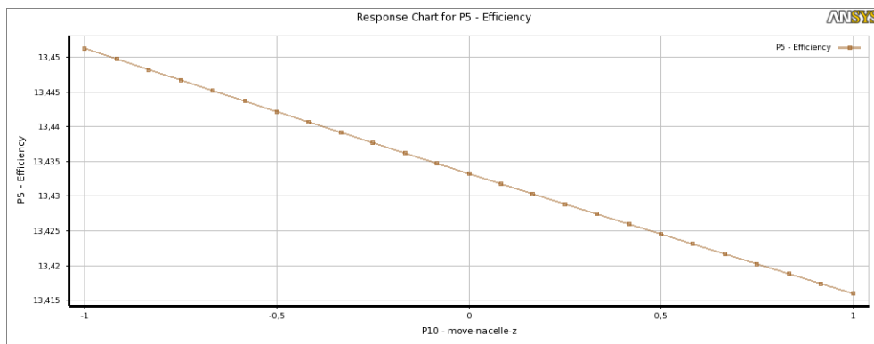
Figure 5.34 – Efficiency vs. z nacelle translation response chart (coarse mesh)
