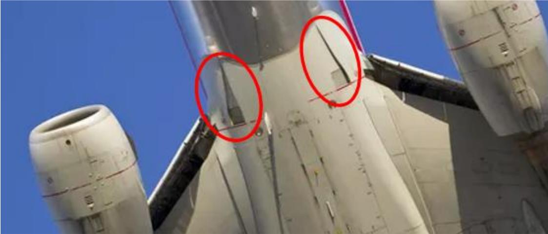
Figure 119: NACA air intakes
