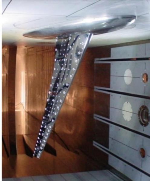
**Figure 32: HIRENASD real model in the wind tunnel**
