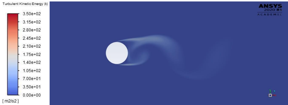
Figure 3.11: Turbulent kinetic energy contour plot ( \Delta t=1 \cdot 10^{-4} s)
