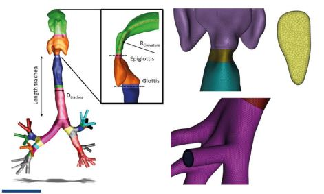
Fig.3. The baseline geometry (left) and its CFD mesh representing a generic patient, ready to receive the parameters of a specific new patient.
