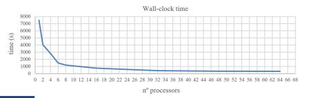
Fig. 5. Clock time vs. number of processors.
