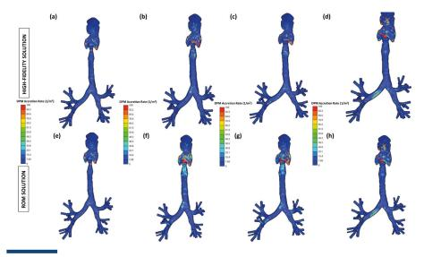
Fig.5. Particle deposition comparison between the high-fidelity CFD simulations (a-d) and the ROM solutions (e-h) for four different virtual patients corresponding to four sets of input parameters.
