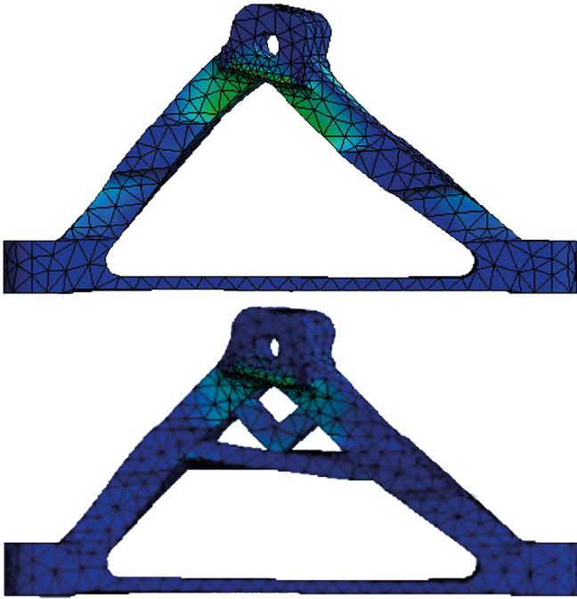
Fig. 10. Bipod short side equivalent stress, before and after optimization.
