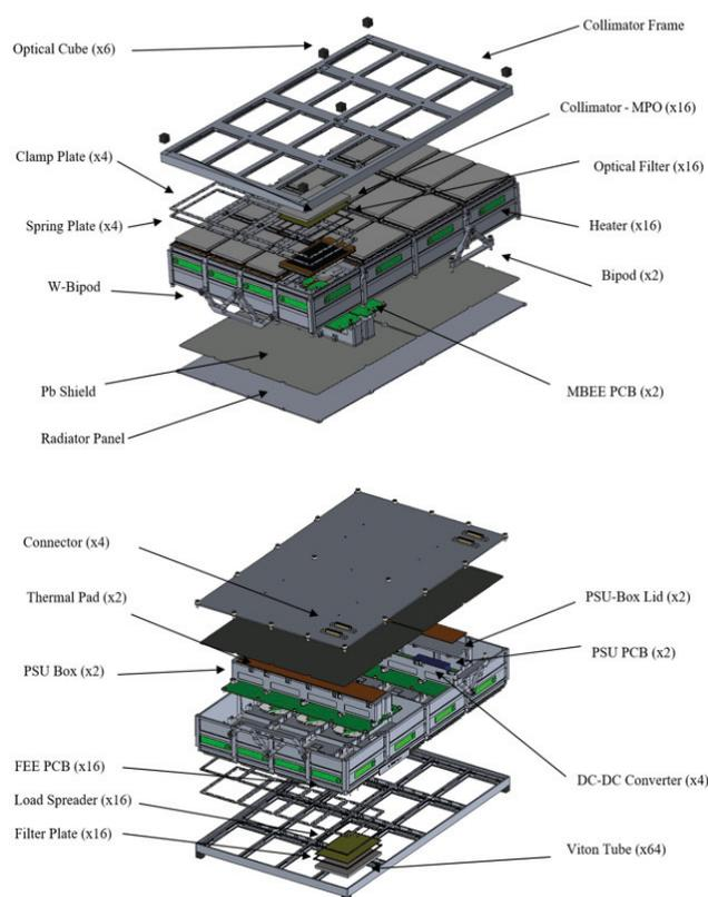
Fig. 2. Exploded view of the module.
