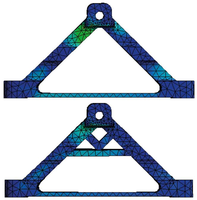
Fig. 11. Bipod short side equivalent stress, before and after optimization.
