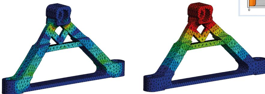
Fig. 7. Optimized equivalent stress.
