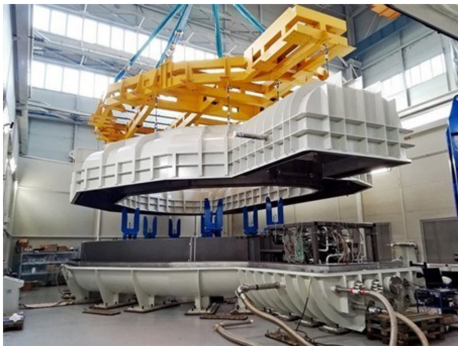
Figure 14: Winding Pack [Retrieved on 21 Jul 2022 on www.fusionforenergy.europa.eu ]
