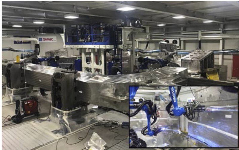
Figure 18: Coil Cases welding [37].
