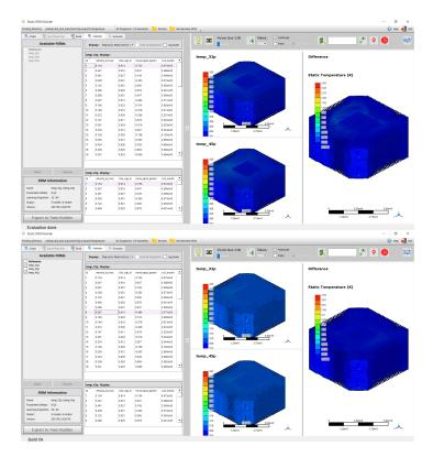
Figure 6.5.13: Temperature comparison between two different snapshots for two ROMs constructed with 32 snapshots and 45 snapshots
