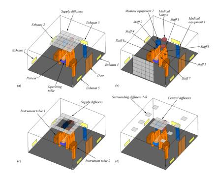
Figure 1.3.4: Description of the several ventilation systems: (a) VLAF, (b) HLAF, (c) DVAF, (d) TAF. Reprinted from Zhai et al. [53]
