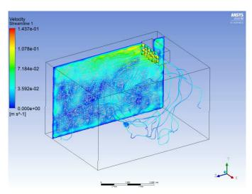
Figure 4.4.2: The figure shows the velocity field on a section of the chamber and HVAC with power lines. The maximum velocity is highlighted in proximity to the exit. HVAC and ceiling case 1#
