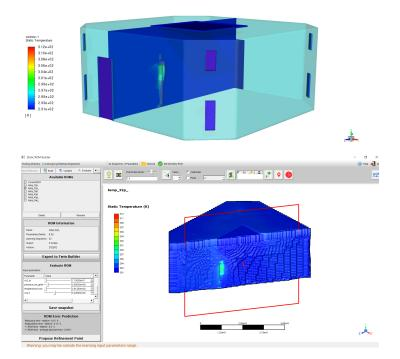
Figure 6.5.14: The two images show on the top the CFD temperature and on the bottom the ROM temperature with 32 snapshots
