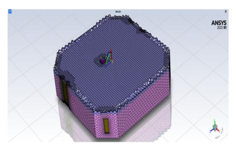
Figure 4.7.1: Operating room geometry discretization: mesh made up of 300k poly-hexa elements.
