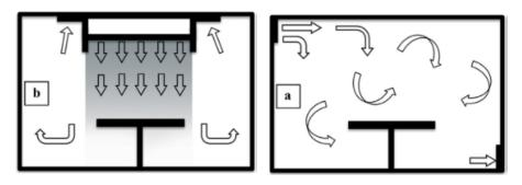
Figure 2.1.1: Figure left is a LAF system, and figure right is a TMA system. Reprinted from Alsved et al. [7].
