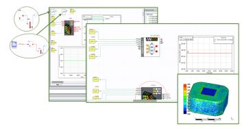
Figure 4.6.1: Twin Builder - FMU model and ROM: results obtained by inserting the ROM or FMU model inside the TB software. The insertion of the input parameter values was highlighted with the circumference and the ellipse.
