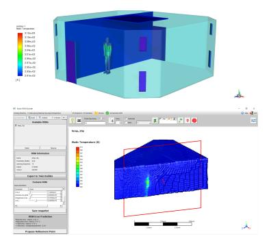
Figure 6.5.3: CFD-ROM comparison: on the top the result obtained through CFD of the temperature field; the bottom figure the ROM with 15 snapshots, with the same values of the parameters used, figure 6.5.1
