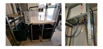
Figure 5.2.5: The figure shows to the left the scale model and three basil used to fill up the tank or to empty it, and to the right, the tank where is highlighted the maximum level of water call as "overfull".
