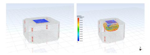
Figure 4.5.1: On the left is the geometry and mesh of the operating room. On the right is represented a transient simulation with particle insertion: inert with two different diameters.
