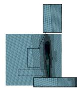
Figure 6.4.4: Case 6c#: detail of the mesh of the operating room and the human dummy.
