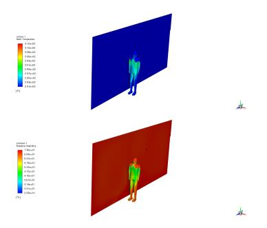
Figure 6.6.5: The temperature CFD field is shown on the top and the related RH field on the bottom.
