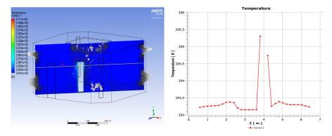
Figure 4.7.3: On the left, temperature field with a superimposed velocity vector field. On the right, the temperature trend in 30 points is extracted along the line on the diagonal section of the chamber.
