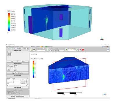
Figure 6.5.16: The two images show on the top the CFD temperature and on the bottom the ROM temperature with 45 snapshots
