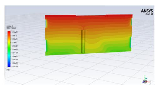
Figure 4.9.5: Trend of the pressure field on the diagonal section of the operating room.
