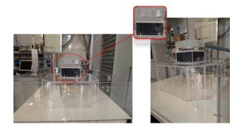
Figure 5.2.4: In the figure is shown the mock-up made of the plexiglass material of the operating theatre. A zoom on the calming baffle is realized
