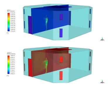
Figure 6.5.2: CFD simulations: on the top figure the result obtained through CFD of the temperature field; on the bottom the result obtained through CFD of the RH field;
