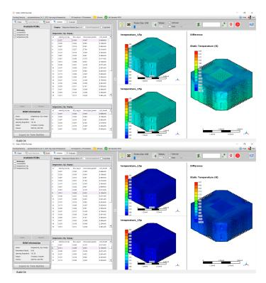
Figure 6.5.8: Temperature comparison between two different snapshots for two ROMs constructed with 15 snapshots and 25 snapshots
