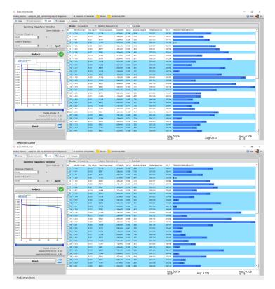
Figure 6.4.7: Top and bottom, two different ROMs built with a different number of snapshots are shown.
