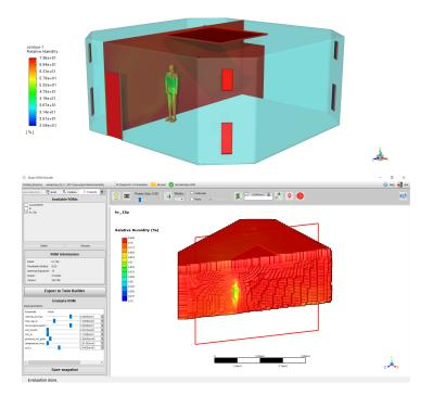
Figure 6.5.4: CFD-ROM comparison: on the top the result obtained through CFD of the RH field; the bottom figure the ROM with 15 snapshots, with the same values of the parameters used, figure 6.5.1
