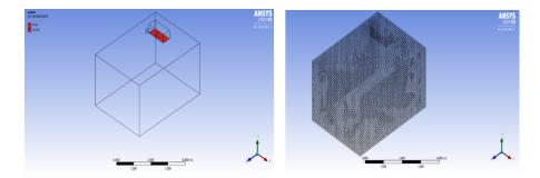
Figure 4.4.1: The figure on the left shows the geometry of a room with an HVAC on which the inlet and outlet of the airflow are indicated. On the right, the same geometry is represented with a mesh with predominantly hexahedral quadrangular elements case #1
