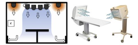
Figure 2.1.2: In figure left, a T<sub>c</sub>AF system reprinted from Alsved[7], and in figure right MLAF system reprinted from Sadrizadeh et al. [78].
