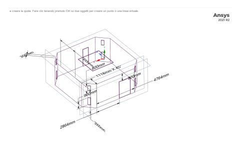
Figure 6.4.1: Geometry of the operating room.
