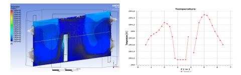
Figure 4.9.3: On the left, temperature field with a superimposed velocity vector field. On the right, the temperature trend in 30 points is extracted along the line on the diagonal section of the chamber.
