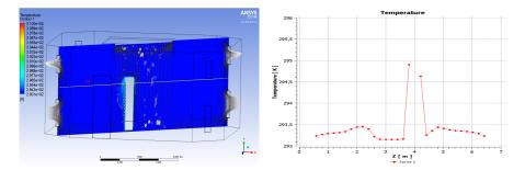
Figure 4.8.3: On the left, temperature field with a superimposed velocity vector field. On the right, the temperature trend in 30 points is extracted along the line on the diagonal section of the chamber.
