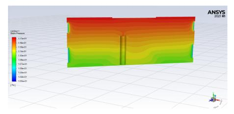
Figure 4.8.5: Trend of the pressure field on the diagonal section of the operating room.
