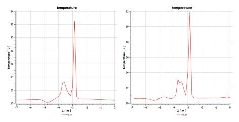
Figure 6.8.8: The chart of temperature extract on the red line (y=1.35m) for two different positions and dimensions of surgical lamps (in evidence): in the left figure (a), the diameter of the lamp is smaller than the one in the right figure (b).
