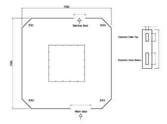
Figure 6.2.1: Geometry of the operating room. Reprinted from Romano et al. [73]
