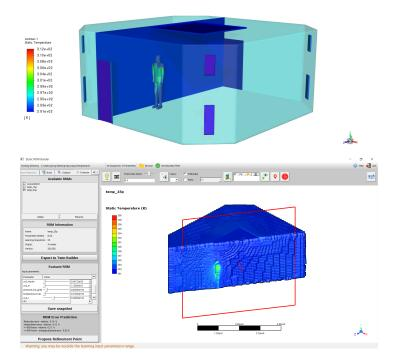
Figure 6.5.5: CFD-ROM comparison: the top figure shows the result obtained through CFD of the temperature field; the bottom figure shows the ROM for 25 snapshots, with the same values of the parameters shown in figure 6.5.1
