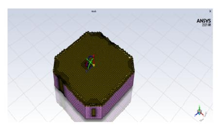
Figure 4.8.1: Operating room geometry discretization: mesh made up of more than 300k poly-hexa elements.
