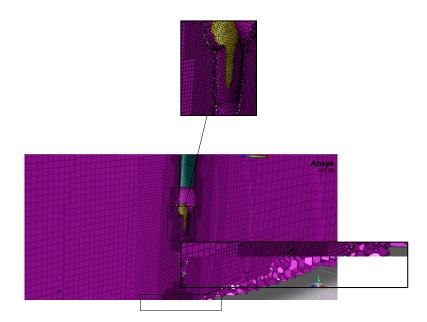
Figure 6.2.4: Detail of the mesh of the operating room and the human dummy.
