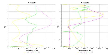
Figure 6.8.11: The chart of velocity extract on the three lines (z=-1.5 yellow line, z=-3.5 green line, and z=-4.5 pink line) for two different positions and dimensions of surgical lamps (in evidence): in the left figure (a), the diameter of the lamp is smaller than the one in the right figure (b).
