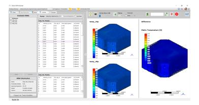
Figure 6.4.8: Difference between two ROMs built with a different number of snapshots.
