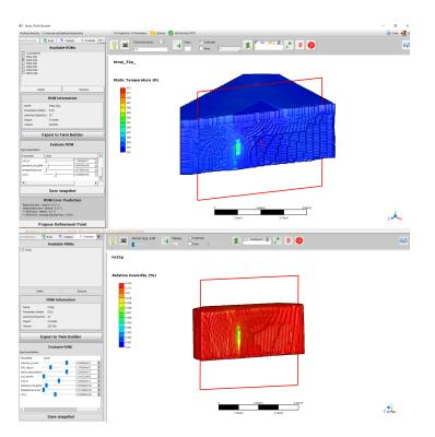
Figure 6.6.6: The ROM related to the temperature field is shown on the top, and the ROM related to the RH field is shown on the bottom.
