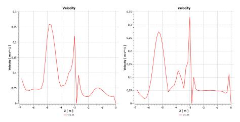
Figure 6.8.10: The chart of velocity extract on the red line (y=1.35m) for two different positions and dimensions of surgical lamps (in evidence): in the left figure (a), the diameter of the lamp is smaller than the one in the right figure (b).
