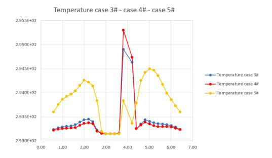
Figure 4.9.7: Comparison between the temperatures obtained in case 3#, case 4# and case 5#. Diagonal section of the chamber on the straight line (a) with coordinates: P1(0.573879, 1.62396, 6.42445) and P2(6.41105, 1.62396, 0.588).
