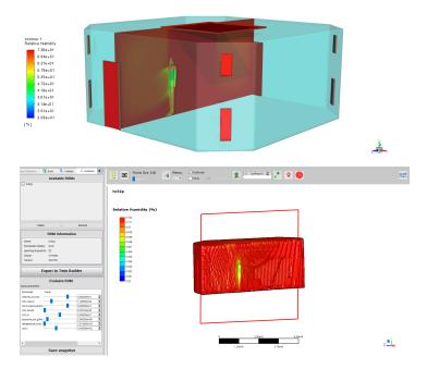
Figure 6.5.15: The two images show on the top the CFD relative humidity and the bottom the ROM relative humidity with 32 snapshots
