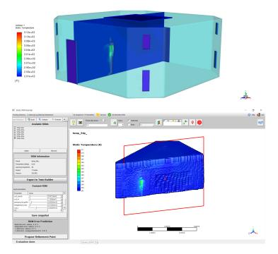
Figure 6.5.17: The two images show on the top the CFD temperature and on the bottom the ROM temperature whit 54 snapshots
