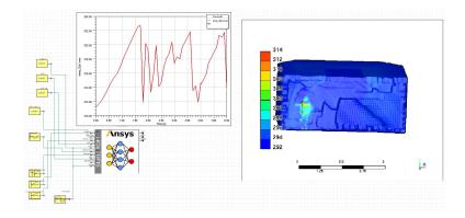
Figure 6.6.3: Operating theatre DT: in the left part, there are the probes of the inlet values; in the right part, there is the ROM and the behavior of average temperature.
