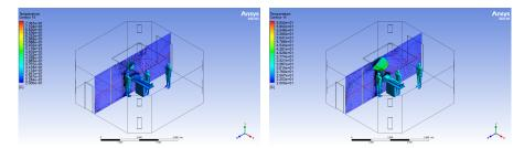
Figure 6.8.9: The temperature slice and vector field of velocity, and four lines to extract the velocity, for two different positions and dimensions of surgical lamps (in evidence): in the left figure (a), the diameter of the lamp is smaller than the one in the right figure (b).
