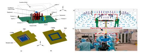
Figure 2.1.3: In the figure left, it is indicated (a) UDF ventilation and (b) Mixing ventilation, Reprinted from Sadeghian[75]. In figure right (a) schematic airflow from a LAF and (b) vertically installed LAF, Reprinted from Sadrizadeh et al. [77].
