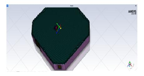
Figure 4.9.1: Operating room geometry discretization: mesh made up of about three millions poly-hexa elements.
