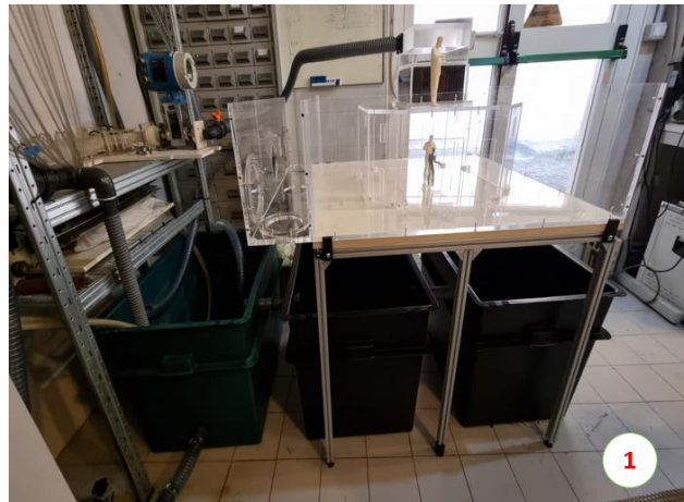
1 The scale model and three basins used to fill up the tank or to empty it 2 The tank where is highlighted the maximum level of water call as "overflow"
