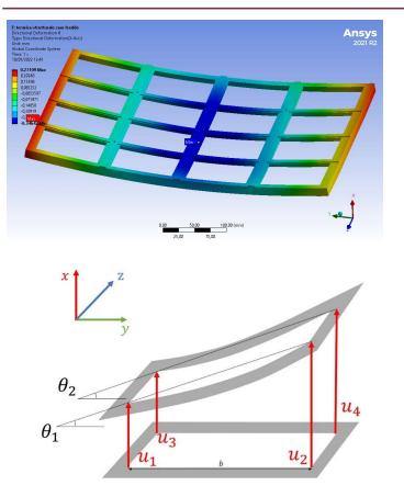
Collimator Frame has been divided into quadrants and the internal longitudinal sides of each quadrant numbered in matrix logic.
