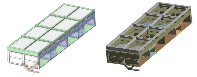
In particular we report the mechanical design, the evaluation of the thermo-elastic deformation of a simplified module, the results of a static structural simulation of a parametric model with an accurate mesh, optimazed throught some mesh morphing tools, the processing and the preliminary optimization of a critical component, the Collimator frame.
