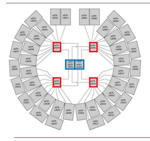
The Large Area Detector (LAD) is designed to be the most sensitive spectral-timing instrument for bright Galactic and extra galactic sources to date, an innovative and highly efficient technology and design allow to deploy in space an effective area as large as 3.2 m<sup>2</sup> - class at 8 keV, adopting a modular configuration.
