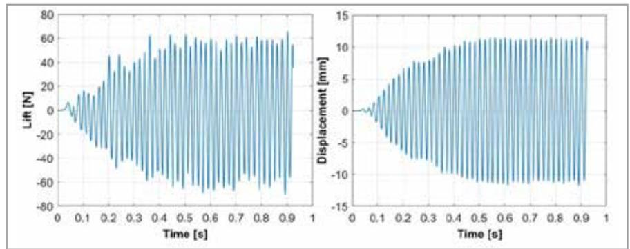
Fig. 7 - Temporal evolution of the lift on the thermowell (left) and the transverse displacement of the tip (right)
