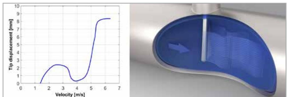
Fig. 2 - Experimental results, RMS tip displacement vs fluid velocity
