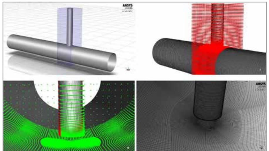
Fig. 5 - RBF Morph configuration to control the embedding of a structural modal shape
