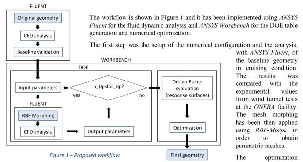
process follows with the computation of the DOE table solution, the generation of the Response Surface and the application of the
