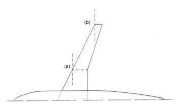
Figure 6 - Axes definition for twisting: (a) kink, (b) tip
