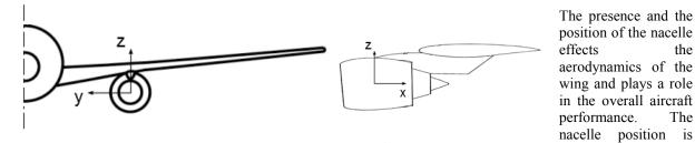
Figure 3 – Nacelle local axes
