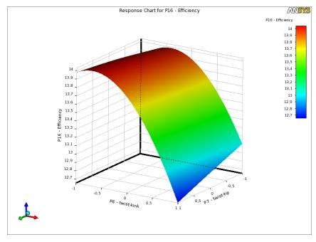
Figure 9 – Efficiency vs. twist kink and tip response surface
