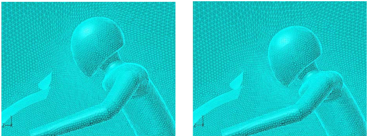
Figure 10: The mesh is morphed to change the driver height (5 cm), note that in this case the 15 deg hunched driver configuration has been used as the starting mesh.
