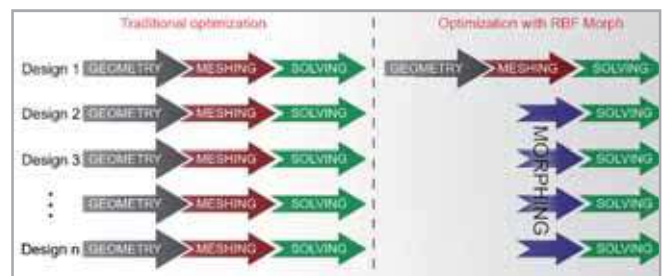
Fig. 1 - Comparison between a traditional optimization workflow and a mesh morphing-based one
