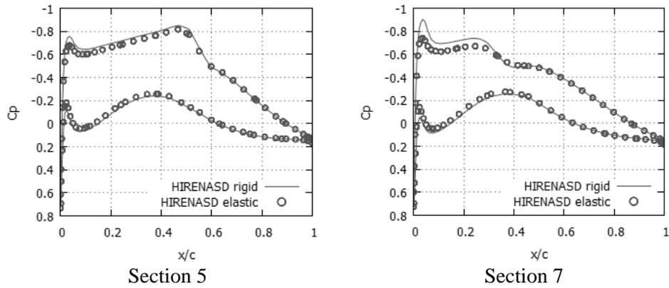
Figure 7. Pressure coefficients for the rigid and the elastic HIRENASD model at different span sections.
