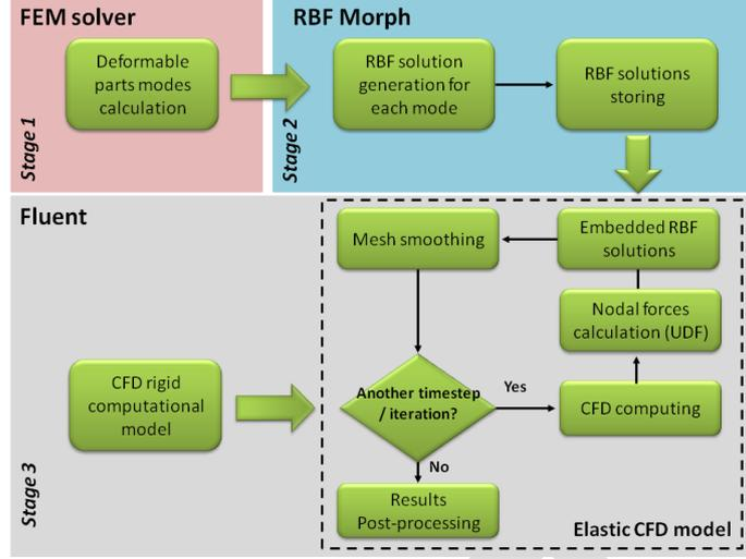
Figure 2. Workflow of the FSI proposed approach
