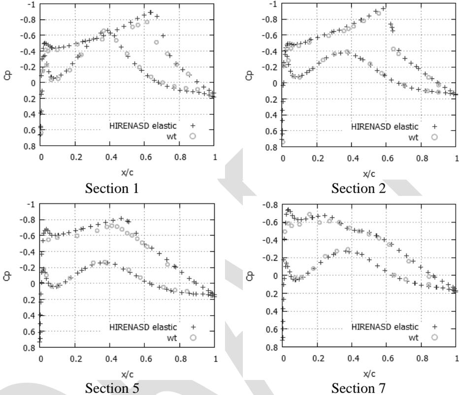
Figure 6. Comparison between numerical and experimental data at different wing sections
