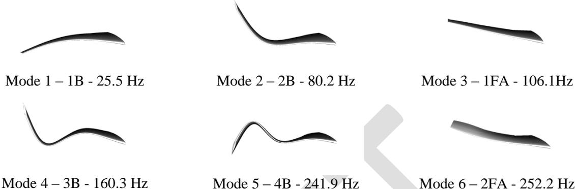
Figure 4. Mode number, description, frequencies and modal shapes for the HIRENASD FEM model
