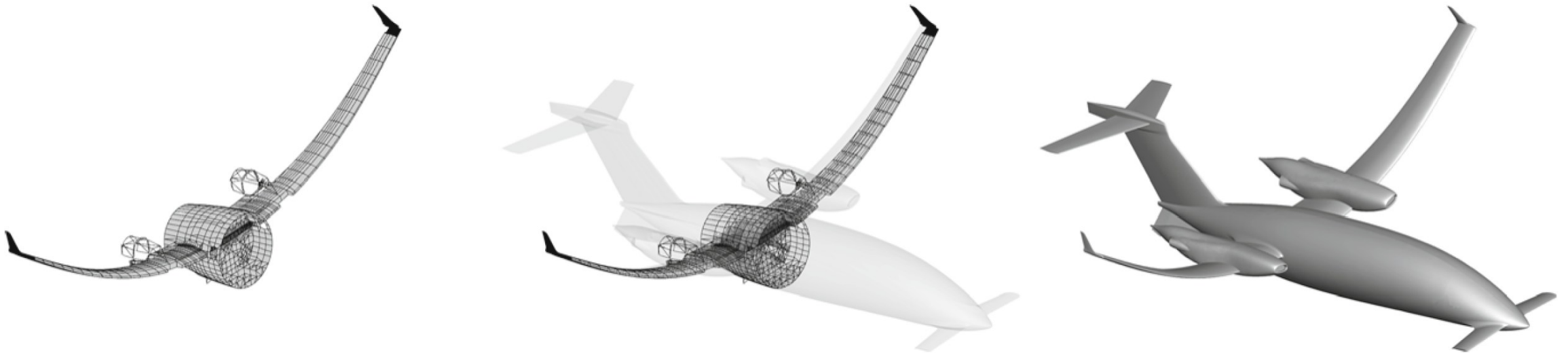
Fig. 7 First structural modal shape and transfer to the CFD mesh
