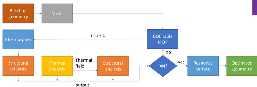
A thermostructural optimization workflow was implemented with 2 parameters changing the length  $L_1$  and  $L_2$  of the u-neck. For each Design Point (DP) thermal and static structural simulation were carried, automatically mapping thermal loads. VM stress, normal stress, displacements, heat to He and component volume as output for each DP and for each step (thermal only, thermal + pressure SBB side, thermal + pressure ICF side). 40 DPs generated with latin hypercube
