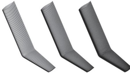
Figure 5: Surface cells clustering for the three levels of grid.
