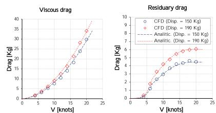
$$D_{H} = \frac{1}{2} \rho_{W} V^{2} S_{wet}(W_{BO}) [(1+k)C_{f} + C_{w}] [1 + k_{\beta} V^{\tau_{\beta}} (W_{BO} + w_{\beta})\beta^{2}]$$
