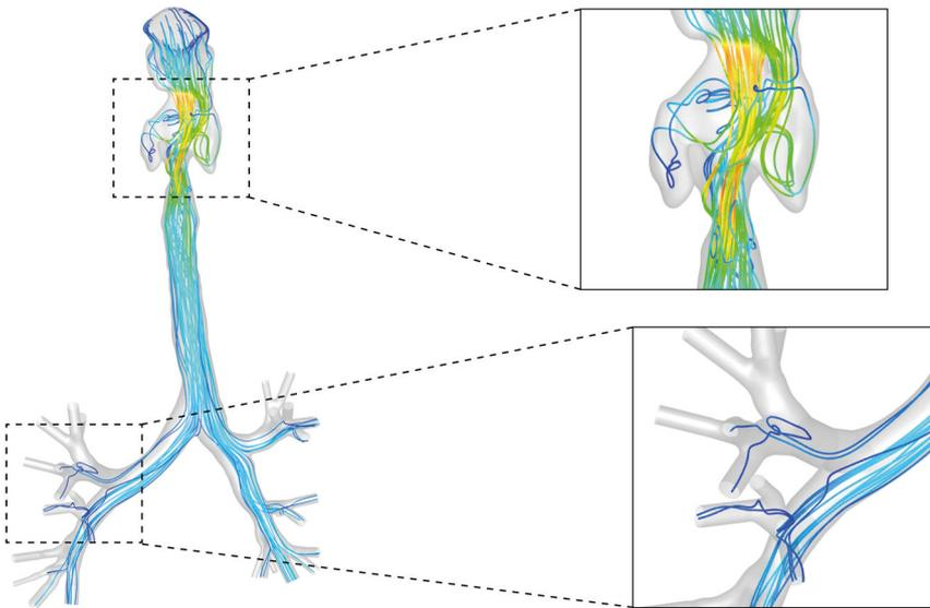
Fig.4. Details of the flow field in a human airway captured by the high fidelity CFD model used in the experiment to represent a generic patient and ready to be adapted to the shape of a specific patient.
