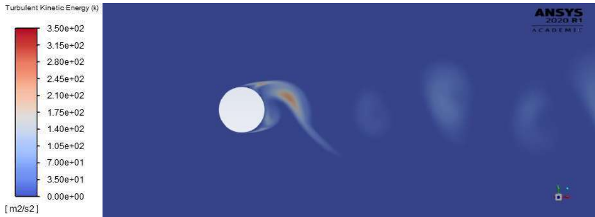
Figure 3.17: Turbulent kinetic energy contour plot ( \Delta t=1 \cdot 10^{-5} s)
