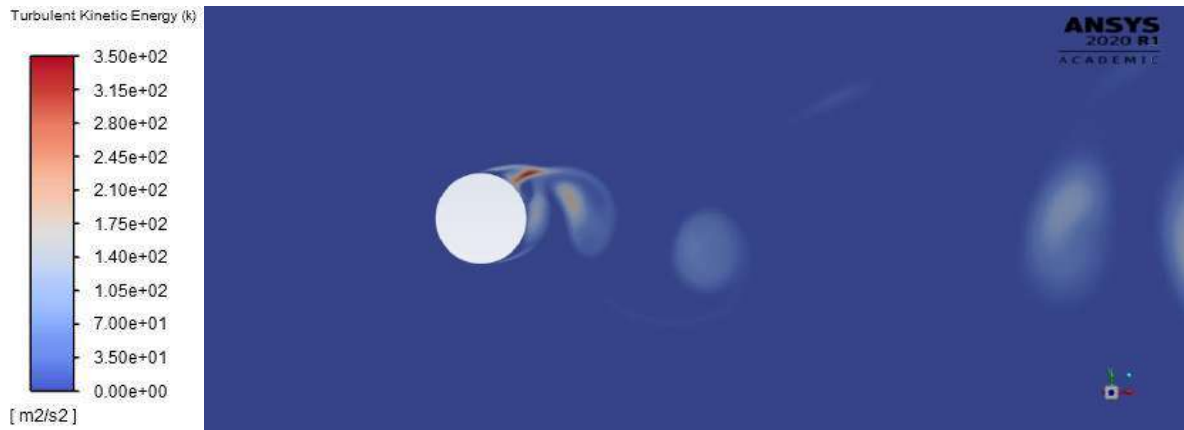
Figure 3.23: Turbulent kinetic energy contour plot ( \Delta t=1 \cdot 10^{-6} s)
