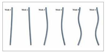
Fig. 4 - First six modal shapes calculated with the FEA model
