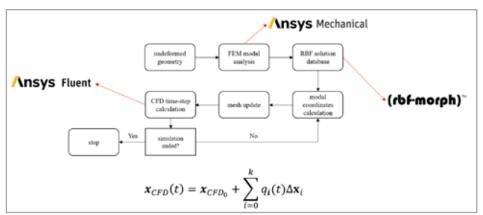
Fig. 3 - FSI workflow based on structural mode embedding by RBF Morph
